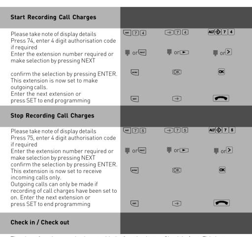
The above function can also be set with the function button Check in / out. This button can be programmed for a specific extension or left empty so that the extension number has to be entered after pressing this button. (See also programming of function buttons)
