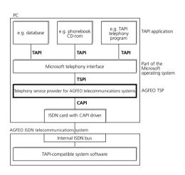
TAPI is an interface of the Microsoft operating system at the application end of Microsoft 's telephone interface. A Telephony Service Provider (TSP) from the manufacturer of the ISDN hardware -in this case AGFEO –is needed to link this to the phone system. The TSP is a driver that must be installed on your PC to run the TAPI functions and to control the necessary exchange of data between the PC and telephone system.
