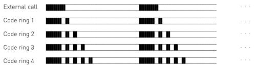
The rings may be different, depending on the terminal equipment in use. The code calls 3 and 4 are not signalled to analog ports that are set to type "radio cell".
