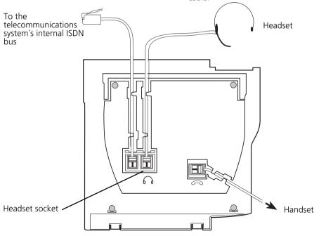
Terminals on the underside of the digital system telephone ST 25
