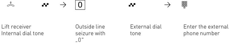
Outside line seizure on the combination port – After the code „10“ has been dialled on the combination port (instead of „0“), the telephone system also seizes an outside line. However, it assigns the fax service to the connection. When an outside line is seized by dialling „0“, the telephone service is assigned.
