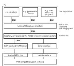
Microsoft's telephony interface. A telephony service provider (TSP) from the manufacturer of the ISDN hardware - in this case from AGFEO - is needed to link this interface to the AGFEO telecommunications system. The TSP is a driver that you must install on your PC. It executes the TAPI functions and controls the necessary exchange of data between the PC and the telecommunications system.
