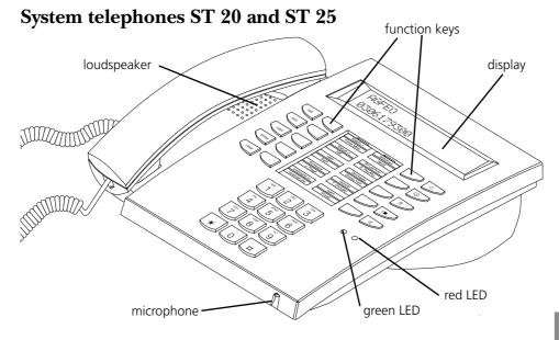
Dialling key pad - For dialling a 1 ... 0 number and entering data
